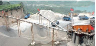
The JOYAL Crushing plant includes vibrating feeder, jaw crusher, impact crusher or cone crusher, vibrating screen, belt conveyor and centrally electric controlling system, etc.
